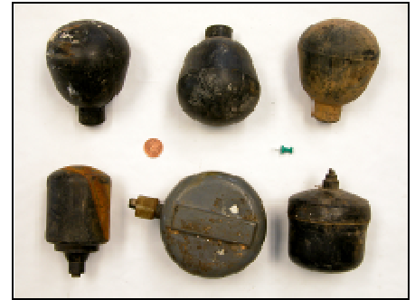
Prohibited: Mercury in level switches
