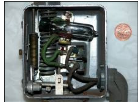
Prohibited: Mercury in pressure and temperature gauges
