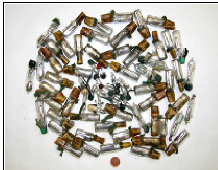
Prohibited: Mercury switches from pressure and temperature gauges
