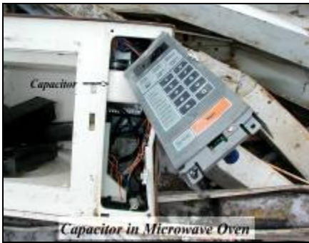
Prohibited: Capacitor in microwave oven
