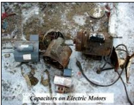
Prohibited: Capacitor in AC motors
