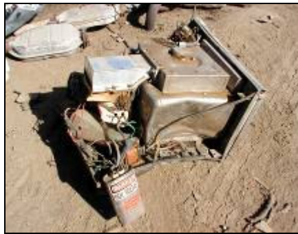
Prohibited: Capacitor in microwave oven
